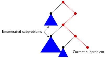
lacktriangle Flashlight algorithm with average delay a and delay d.
